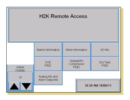
H2K Remote Telemetry can be accessed via a Remote Access System that allows full remote control of the treatment process real time via Cellular Internet Connection. No software is required for this operation. Connection via any internet browser and some smart phones is all that is required.
